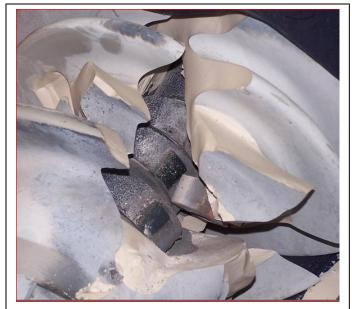
Figure 16 Always take great caution when handling fractured porcelain, the edges are razor sharp
