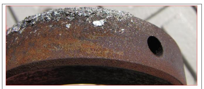
Figure 6 An internal steel component of a porcelain housed arrester that shows old and new rust along with molten metal over the old rust
