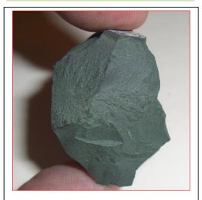
Figure 15 Section of disk chipped out for testing without influence of faulted section
