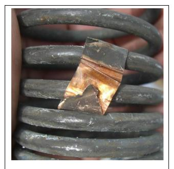
Figure 8 Shinny copper shunt implies no moisture ingress or excess partial discharge
