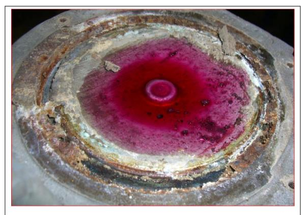
Figure 9 Red Die penetrating fluid can be very useful in locating cracks or pinholes in metal diaphragms
