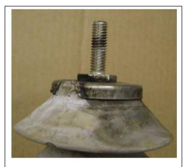
Figure 11 Arrester where external flashover did not fail the arrester, but damaged the seal
