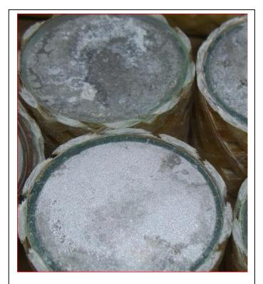
Figure 10 Evidence of Moisture in a solid core polymer housed arrester. Oxidized aluminum
