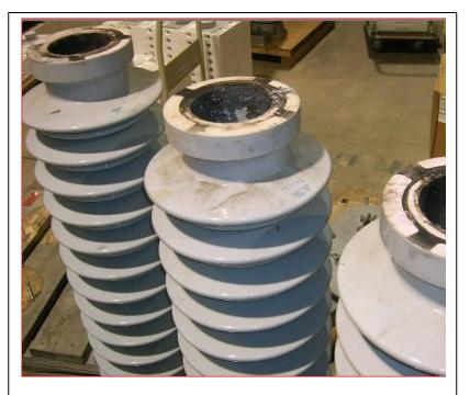
Figure 1 Porcelain Station Arresters with internal core that has experienced a fault current event
