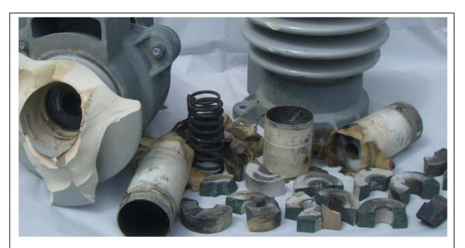
Figure 5 All too often Overload or Failure mode of Porcelain Station Arresters
