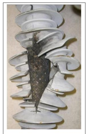
Figure 4 Example of Non-fragmenting nature of polymer housed arresters upon overload or failure
