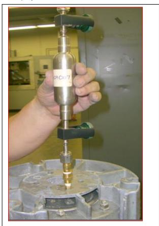
Figure 2 Taking a gas sample of an unvented companion arrester can be very useful in the analysis
